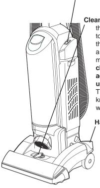
Cleaner Height Setting. An adjustment that raises or lowers the cleaner base to match the type of floor surface. With the cleaner cord unplugged, set the adjustment to lowest setting for maximum carpet cleaning. If the cleaner is difficult to push, move adjustment to next highest setting until cleaner is comfortable to push.
